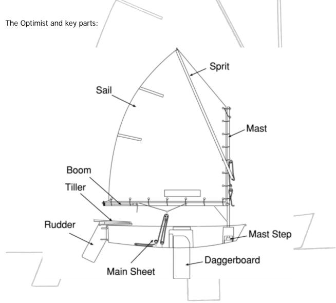
This manual includes the fitting and preparation of the following parts of the Optimist:
